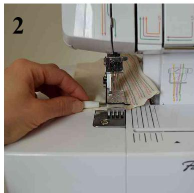
3. Hold down the needle thread tension release buttons while you use the tool to pull the needle threads out to the front edge of the machine.
